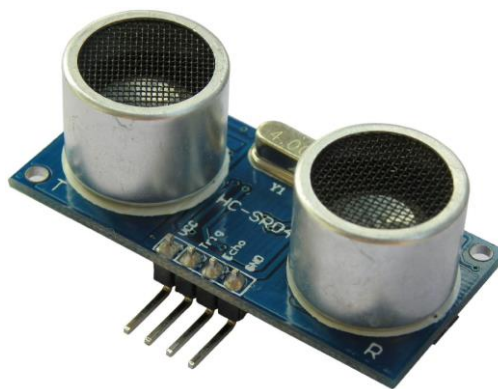
Figure 6 HC-SR04 Ultrasonic Sensor
